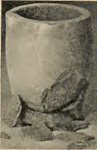
Fig. 36—A scalped crucible
